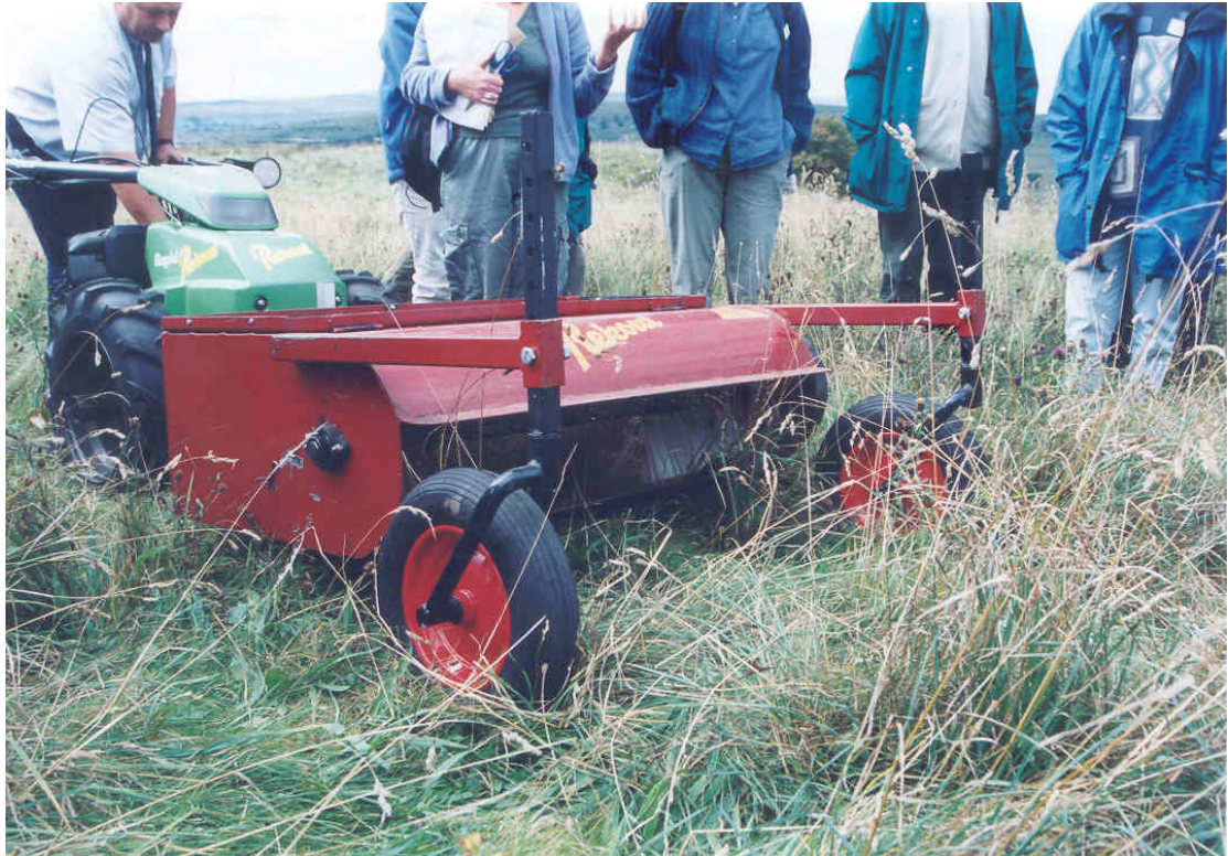
The front mounted Rekord seed harvester.
