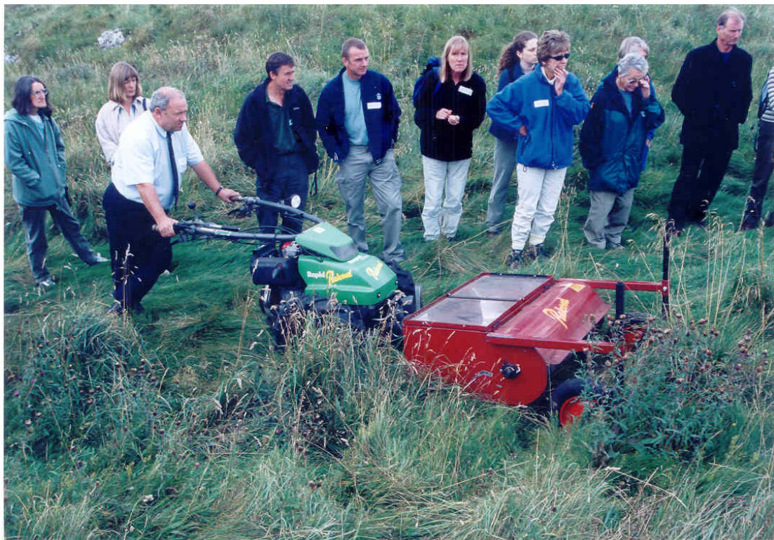
This machine is designed to drive a range of front mounted equipment including cutting and baling machines. It is used in upland Continental hay meadows on difficult terrain.
